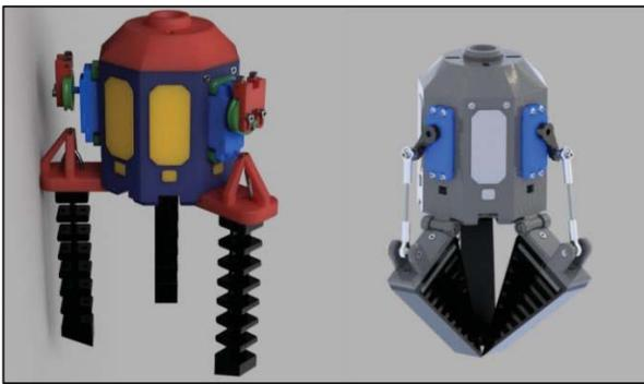
Fig. 3: Gripper design - Concept TDD (left); Concept CDD (right)
