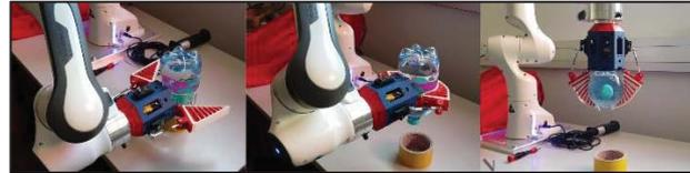
Fig. 4: Successful grip of a 1L bottle with the CDD concept
