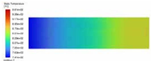
Figure 9 - "NG" Case - Temperature of the steel strip (scaled)
