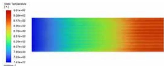
Figure 10 - "H<sub>2</sub>" Case - Temperature of the steel strip
